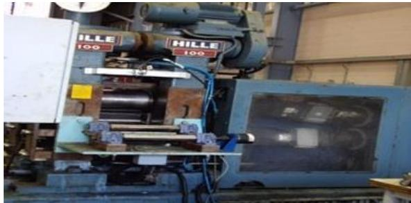
Figure 1. Hille 100 rolling mill
